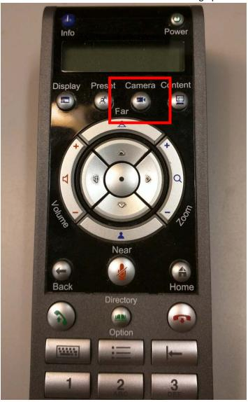
2. Select your camera input. Your conference room may have multiple cameras. Typically, the main camera is attached to camera input1. The Background image will be a preview of the from that camera input. In the Example Below, the camera is connected to camera input 1.
